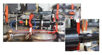
Figure 1. A Sequoia Scientific LISST-HOLO holographic camera was plumbed into the ship's seawater delivery system for the transit across the Drake Passage. The flow was sampled before bubble removal and after the flow passed through a coarse mesh that prevented large particles from making it to the camera.
