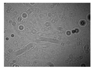
Figure 2. The LISST-HOLO holographic camera measures the diffraction interference pattern created from forward light scatter from all particles suspended within the sample volume.
